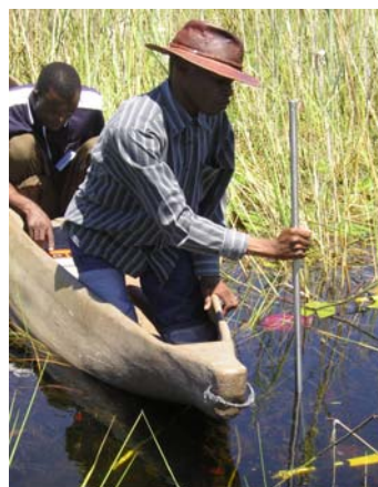
Course participants Golden Msilimba and Batsile Bathusi measuring stream velocity using a velocity probe in the Okavango Delta
