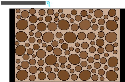
A soakaway pit is a simple structure made by digging into the ground, and then lined or filled with gravel stones. The stones in the soakaway pit allows the dirty water (greywater) to drain into the surrounding soil and minimises our contact with the dirty water.
