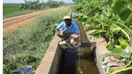
Flow measurement in open canals using current meter
