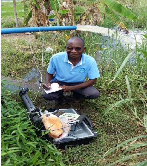
Flow measurement in pipes using ultrasonic flow meter
