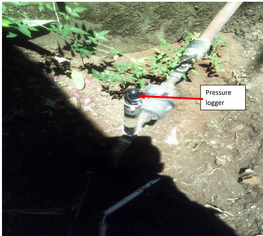
Figure 3: Pressure logger installed on customer meter to measure pressure for 7 days.
