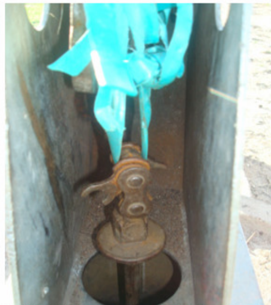
Plate 4-6: Broken down HP with its rods sustained by a piece of bicycle chain and manila rope
