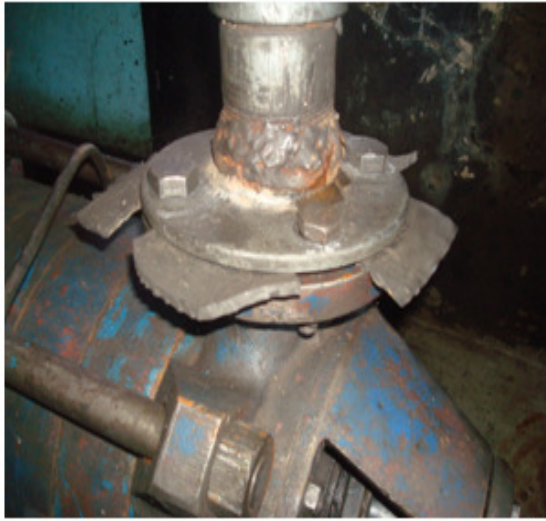
Plate 4-3 and 4-4: Forged spare parts and the threaded Joint is welded at Kibara Scheme
