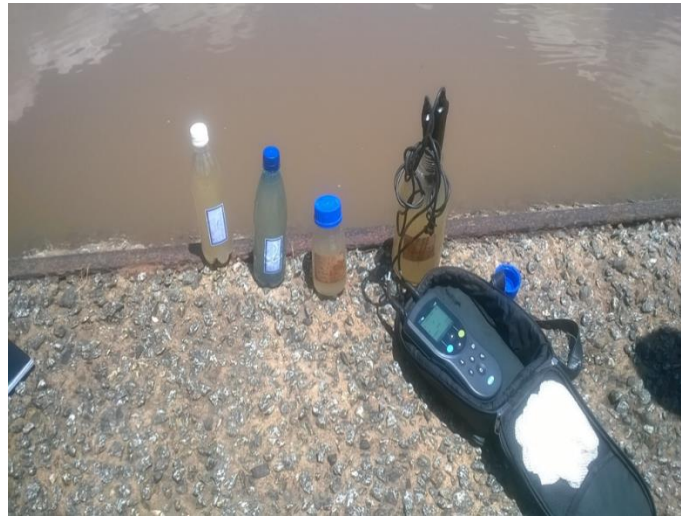
Figure 2: Hach PC Multi Direct Multimeter
