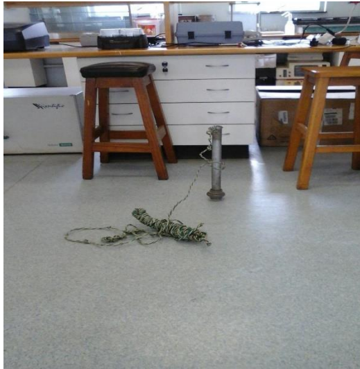
Figure 1: Surface Water Sampler (DWA)
