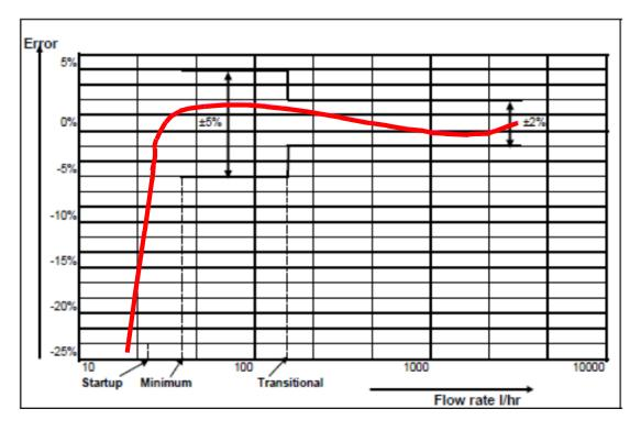
Figure 2.3: Customer meter error curve (Adopted from Harawa et al, (2015))
