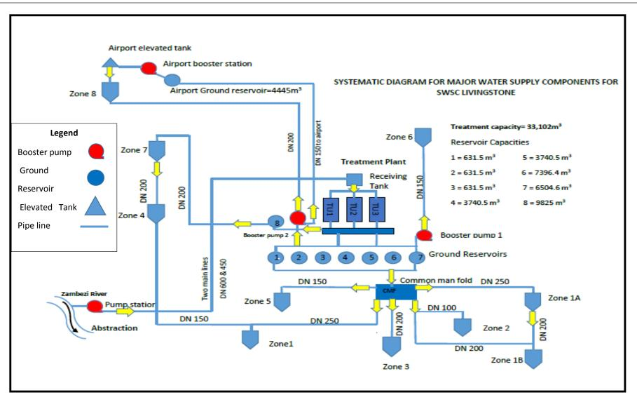
Figure 3.2: Systematic diagram for major supply components
